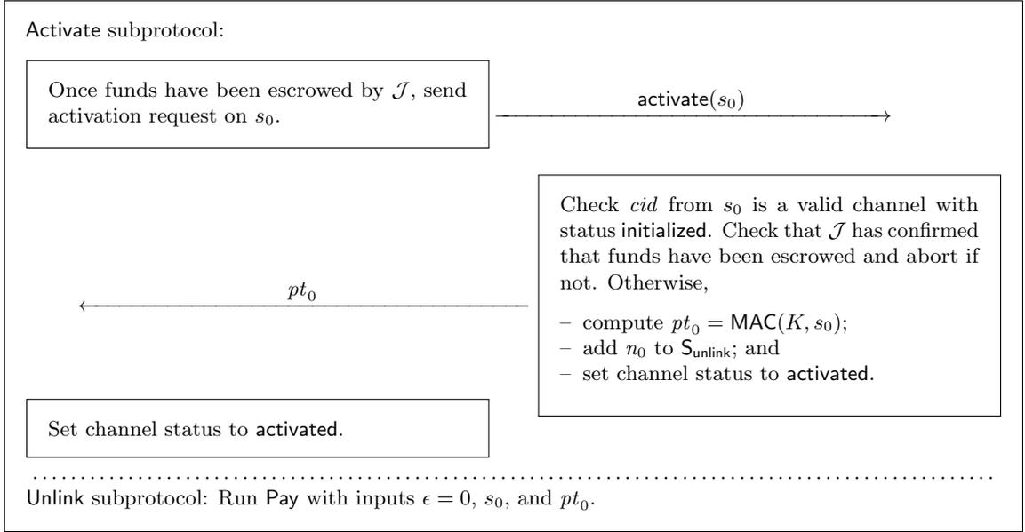
**Figure 5.3:** 2PC Establish protocol with UTXO-based arbiter: **Activate** and **Unlink**.
